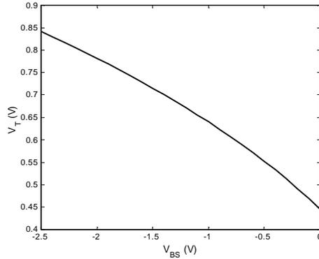
Figure 3.14 Effect of body-bias on the threshold.
