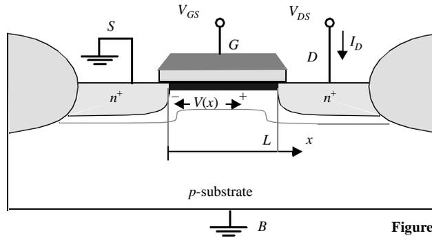
Figure 3.15 NMOS transistor with bias voltages.
