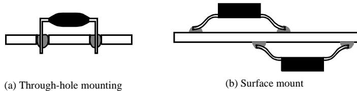
Figure 2.14 Board-mounting approaches.
