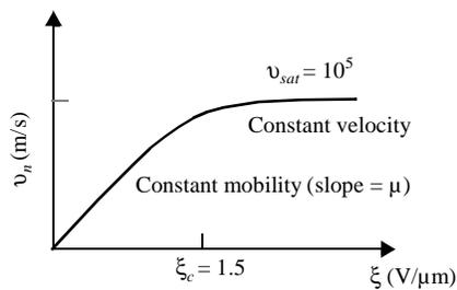
Figure 3.17 Velocity-saturation effect.
