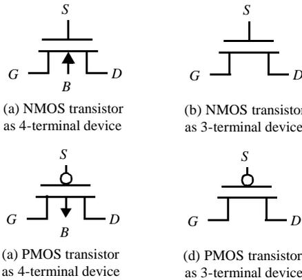
Figure 3.12 Circuit symbols for MOS transistors.
