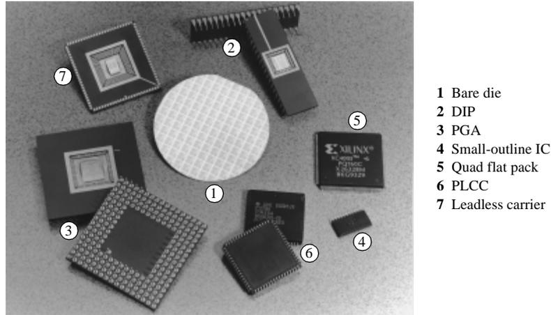
**Figure 2.15** An overview of commonly used package types.
