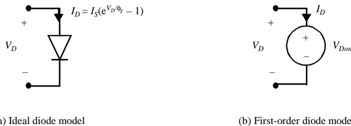
Figure 3.6 Diode models.
