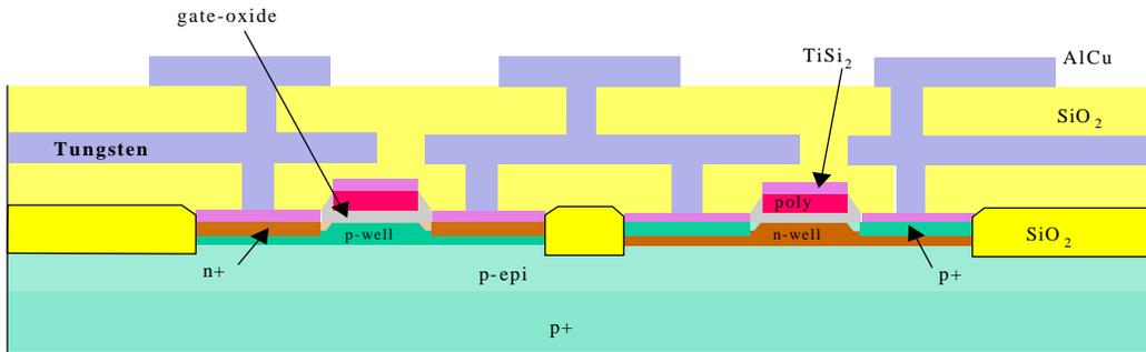
Figure 3.11 Cross-section of contemporary dual-well CMOS process.
