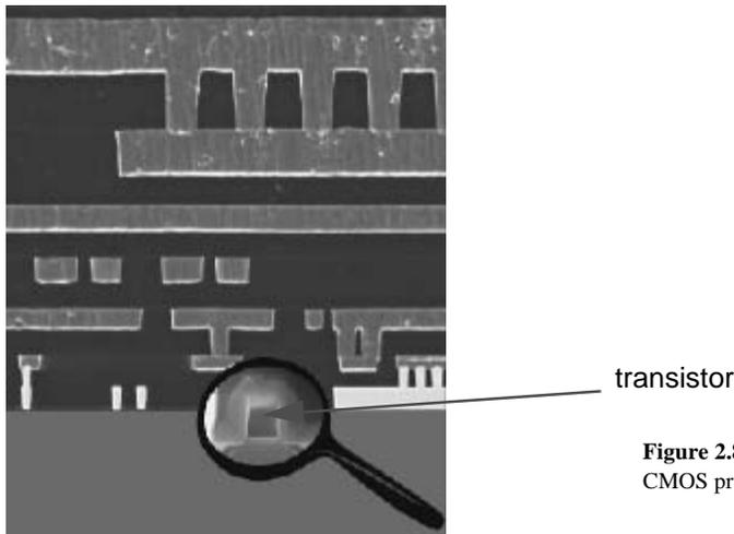
**Figure 2.8** Cross-section of state-of-the-art CMOS process.
