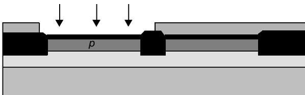
(f) After  $p$ -well and  $V_{T_n}$  adjust implants
