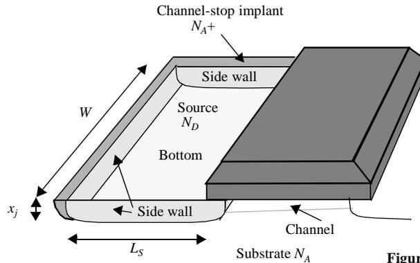
**Figure 3.32** Detailed view of source junction.
