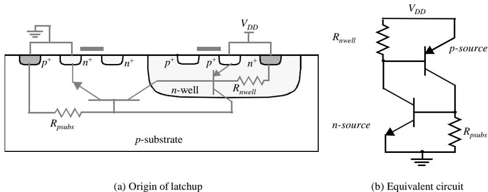
Figure 3.37 CMOS latchup.
